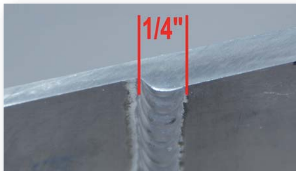
Weld Must Be 1/4 Inch Wide
