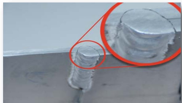
Weld Must Have Deep Penetration
